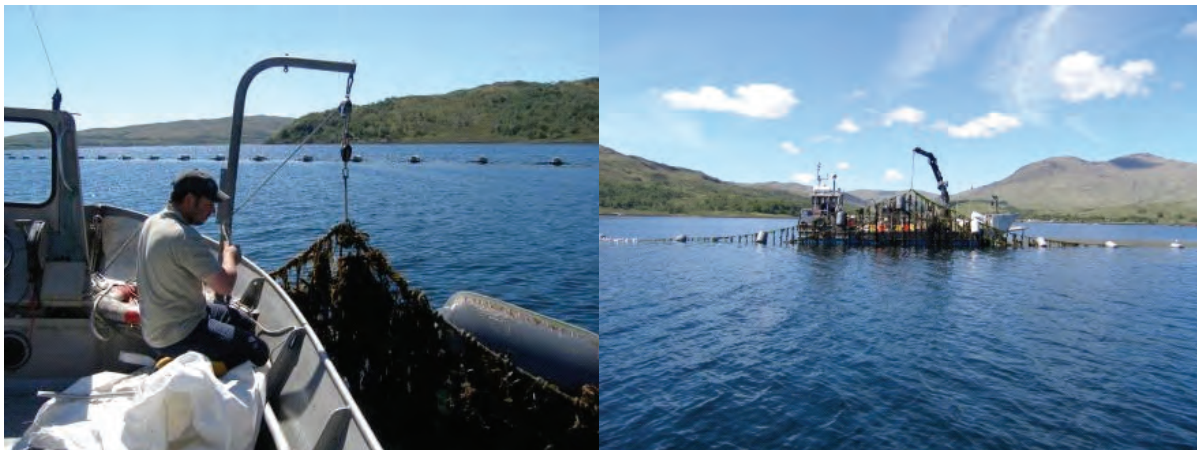
Figure 3. Two types of boats used in the different stages of sampling, on the left the small boat with a small crane used mainly during inspection, and on the right the largest boat, with a large crane used mainly for harvesting and socking processes.
