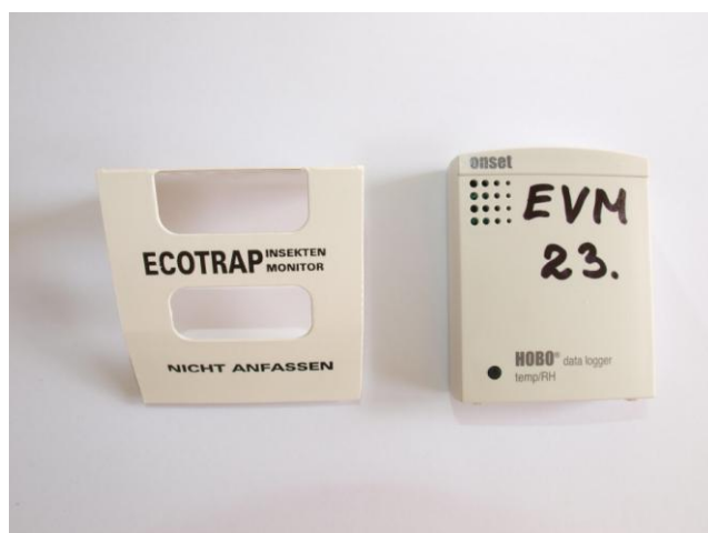
Fig. 1. Temperature and relative humidity logger (on the right), sticky trap (on the left)
