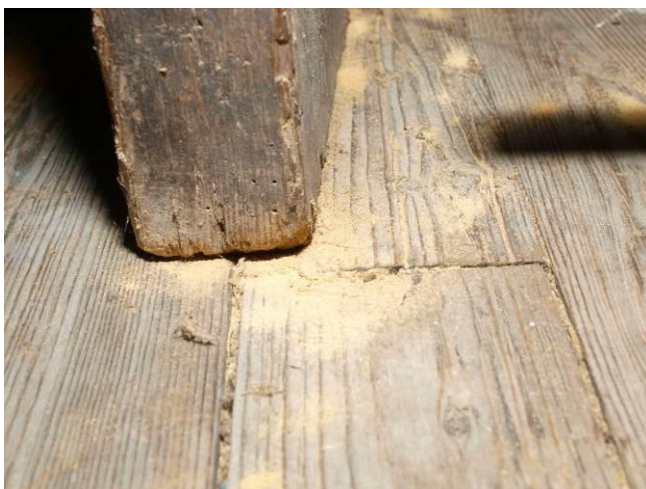
Fig. 9. Bore dust all around handlooms, which indicates active attack
