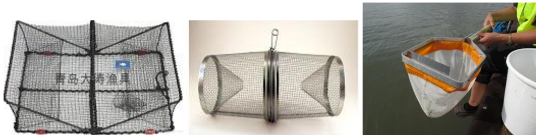
Figure 2. Sampling equipment used in the alien species survey (from left to right): Chinese crab trap, Minnow fish trap and scraping tool (HELCOM 2012).
